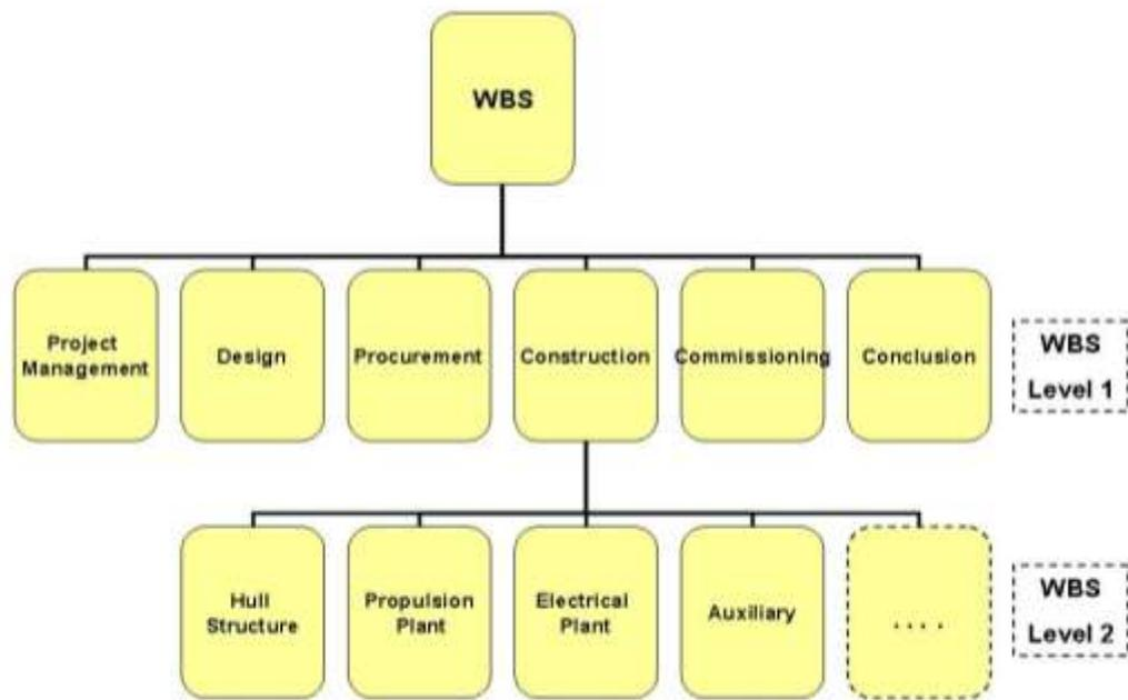
Figure 1: Typical Work Breakdown Structure – WBS
