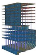
81 panels 24 pillars Aft ship section [A]
