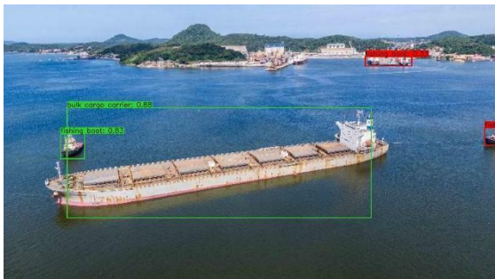
Figure 12 – Bulk cargo carrier detected through deep learning with a confidence score of 0,88
