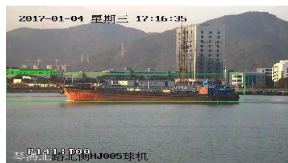
Figure 4 – Bulk Cargo Carrier detected through deep learning with a confidence score of 0,99
