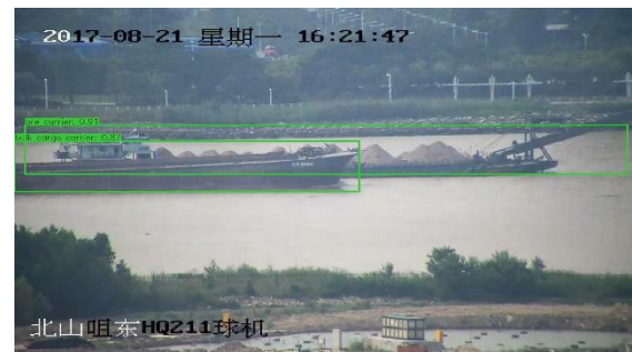
Figure 10 – Ore carrier has a confidence score of 0,91 and Bulk cargo carrier has a confidence score of 0,87 under occlusion detections
