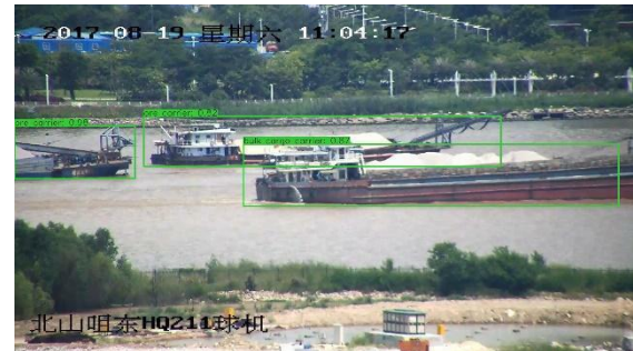
Figure 9 – Ore carriers under occlusion detected through deep learning. The ship on the left has a confidence score of 0,98, the ship in the middle has 0,82 and the ship on the right has 0,87.
