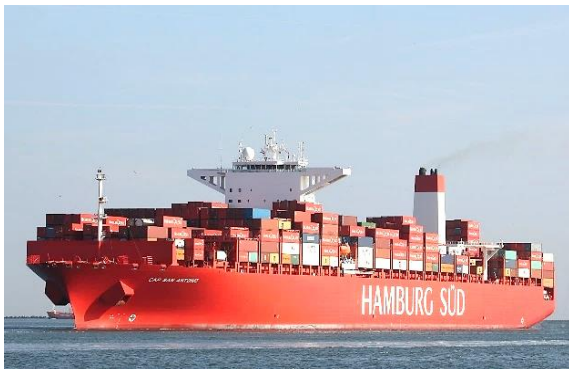
Figure 2: Cap San Antonio (IMO:9622241): Gross Tonnage: 119441; Overall Length (LOA) 333.2 m; Breadth Extreme: 48,32 m; Loaded Draught: 14,2 m; construction year 2013/2014; Design Speed: 22 knots (MARINE TRAFFIC, 2020)
