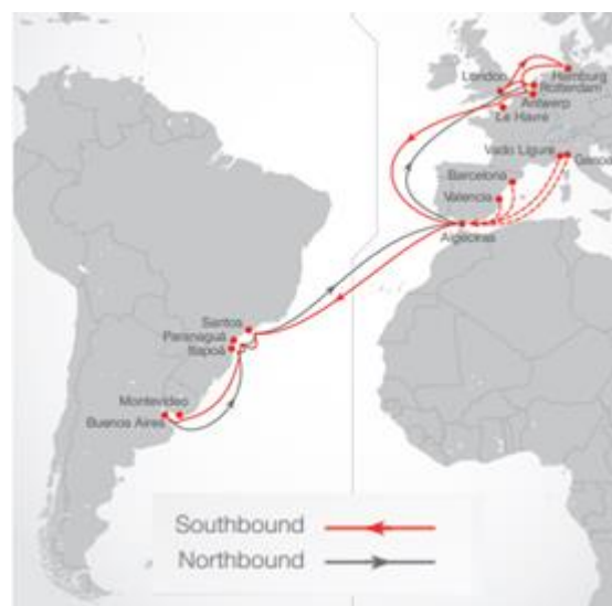
Figure 1: Aliança Line Service Route (SAEC1) operated by eight same class Post-Panamax vessels within up to 9814 TEUs of Nominal Capacity, calling weekly at 14 ports in 56 days round trip on average, on Northbound and Southbound directions.
