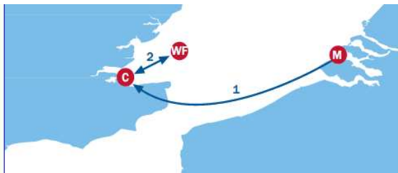
Fig. 4: Second strategy to install OWF where “WF” means Wind Farm, “C” means Center for storage and pre-assembly and “M” means Manufacturing
